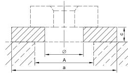
Load transfer plate 1) for angle compensation tube TR 2150-Ø
