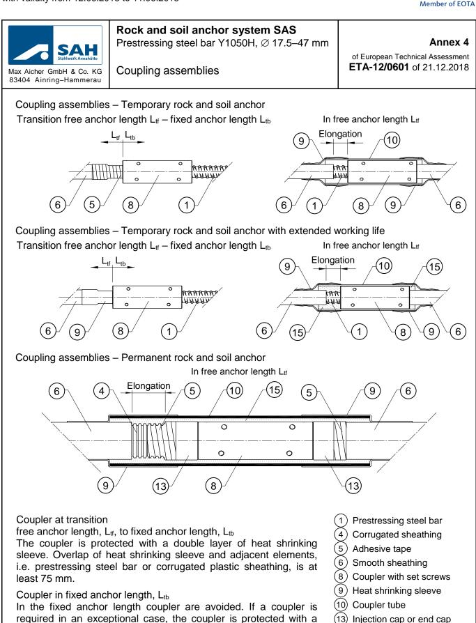
(15) Corrosion protection grease sleeve and adjacent elements, i.e. prestressing steel bar or corrugated plastic sheathing, is at least 75 mm.
