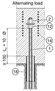
Permanent pile with sheathing according to EN 1537
